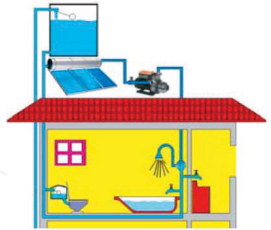
Hot water boosting in solar heating system
