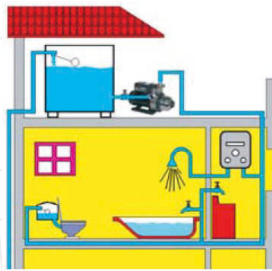
Indirect roof tank water pressure boosting
