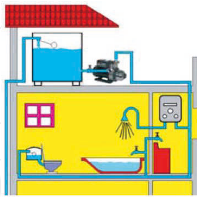
Indirect roof tank water pressure boosting
