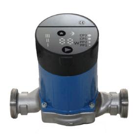
ECT-AHW & ECT-AHWS series is a high energy-efficient variable speed circulator pump, this series pumps provide 8 different modes selection, such as Highest / Lowest proportional pressure, Highest / Lowest constant pressure, Highest / Medium / Lowest constant speed, and Night version to replace existing fixed speed circulators in order to meet most circulation systems.
